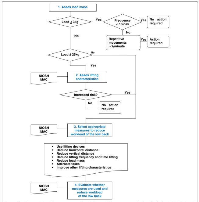
Figure 1 Flow chart consisting of four steps to assess the risk of manual lifting to prevent work-related low back pain (NIOSH: National Institute for Occupational Safety and Health lifting equation, MAC = Manual handling Assessment Charts-tool).
