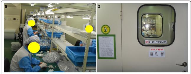
**Figure 1 Cleanroom workers inside the cleanroom. a.** Inside the cleanroom, workers are assembling with components of endoscopic devices with chloroform adhesives. **b.** The cleanroom is covered up tightly.
