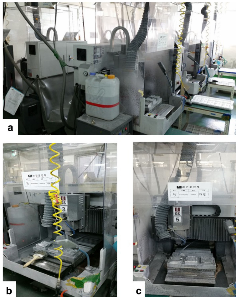
Fig. 2 a CNC machines were arranged in a row. About 30 machines operated on duty. A plastic drum which did not have any hazard marker contained methyl alcohol. b and c CNC machines were always open. Gray rubber hose was ventilating system. However, these did not operate properly
